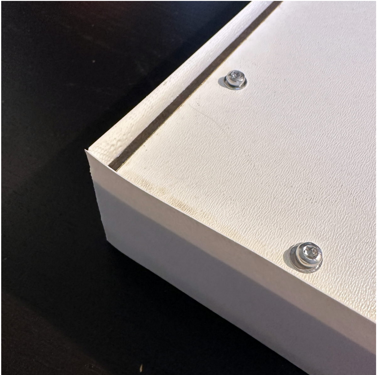
Fig. 13: Edge band applied before cutting off excess.
