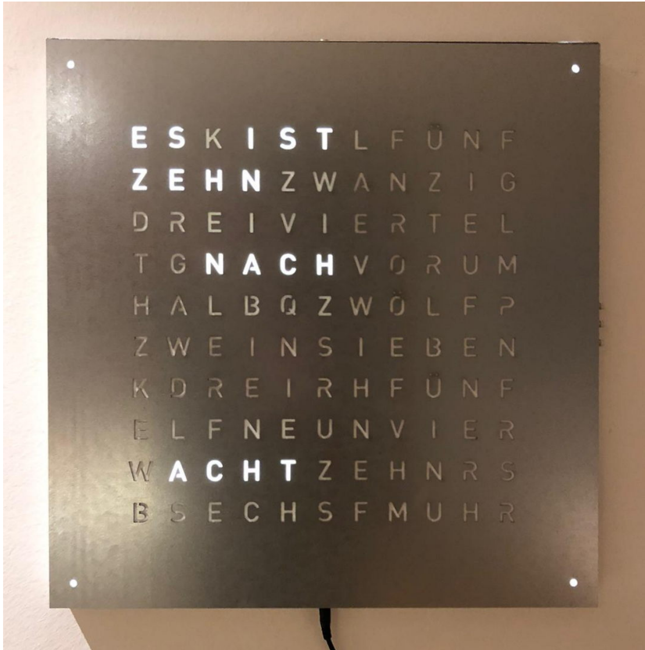
Fig. 2: OpenWordClock with laser cut zinc steel front panel. A polystyrene diffuser evens the illumination of the letters.
