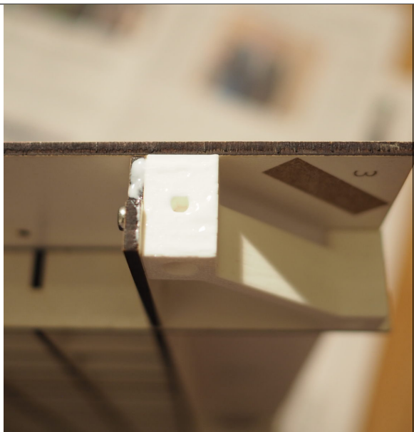
Fig. 11: Wood glue applied on corner block.
