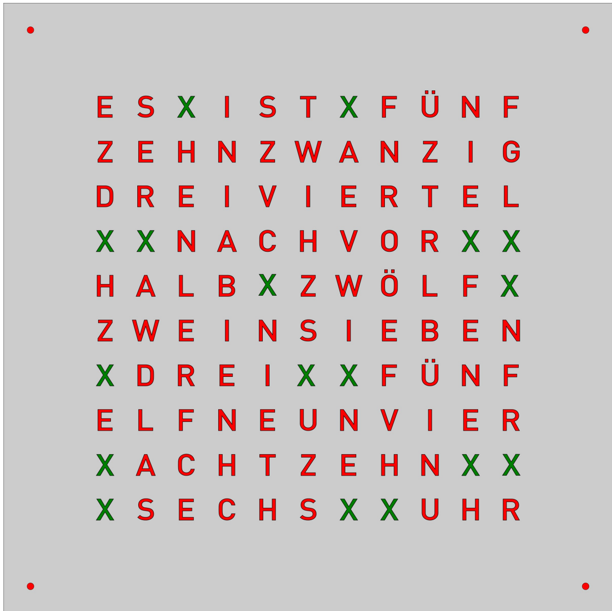
Fig. 21: A possible letter placement on the front panel for the OpenWordClock. The red letters need to be positioned as shown and allow only for very little variation. The green “X” are filled with random letters.
